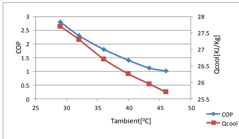
**Figure 4.** Recirculation mode ( COP vs T<sub>amb</sub> vs Q<sub>cool</sub>)
