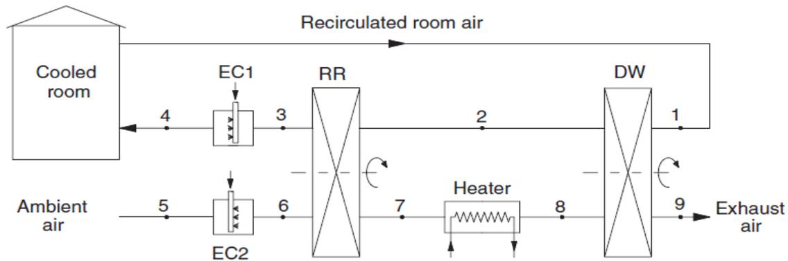
**Figure 2.** Schematic diagram of desiccant cooling system in regeneration mode (M.Kanoglu *et al.*,2007)
