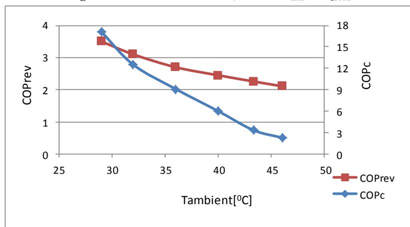
**Figure 5.** Ventilation mode ( COP<sub>rev</sub> vs T<sub>amb</sub> vs COP<sub>c</sub>)
