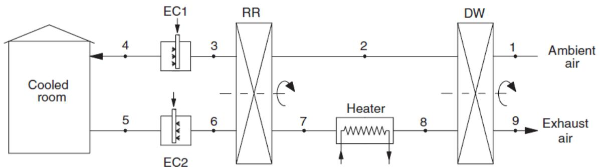
Figure 1. Schematic diagram of desiccant cooling system in ventilation mode (M.Kanoglu *et al.*,2007)
