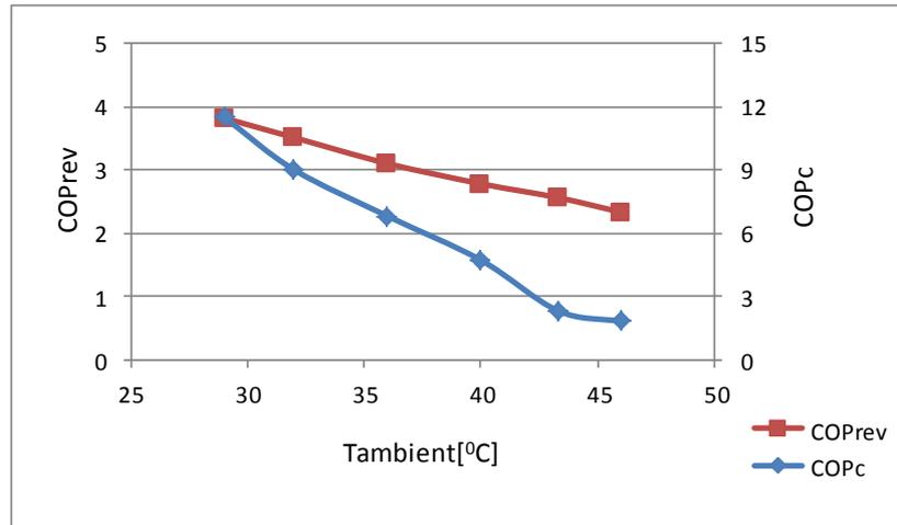
**Figure 6.** Recirculation mode (  $COP_{rev}$  vs  $T_{amb}$  vs  $COP_c$ )
