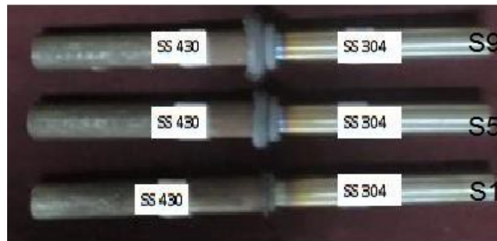
Figure 2. Samples of Friction welded joints.
