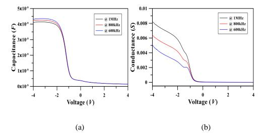
**Figure 1**. **a**) Capacitance and **b**) Conductance characteristics vs voltage of Al/ PbO/ *p*-Si for 600kHz, 800kHz and 1MHz.
