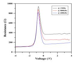
**Figure 3.** The voltage - dependence of  $R_s$  at 600kHz,
