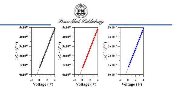
Figure 2. C<sup>-2</sup>-V plots of Al/ PbO/ p-Si a) at 1MHz b) at 800kHz and c) at 600kHz.
